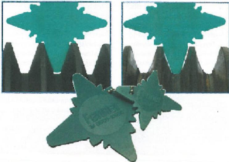
This is a picture of the pulley go/no go gauges that we have provided, as you can see these give you an immediate indication if your pulleys need to be replaced before new belts are fitted.
