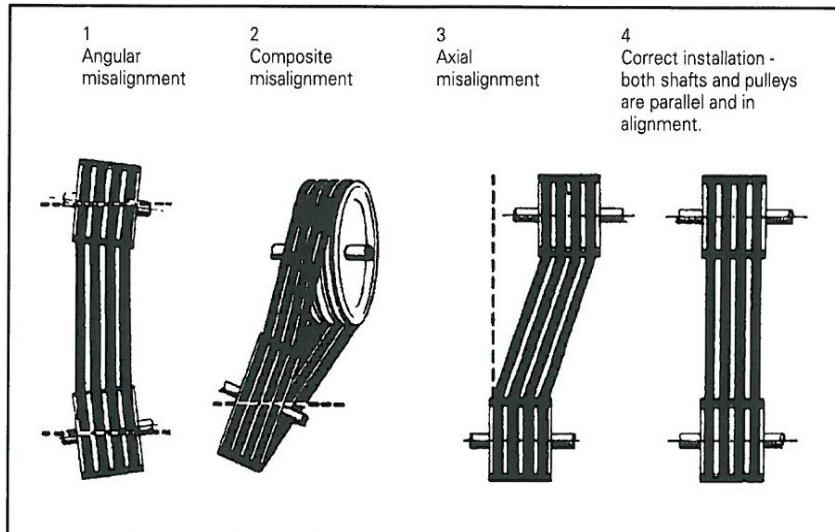
As you can see from the diagram it is detrimental to the belts that the alignment is correct. If the alignment is not correct the pulleys and belts will suffer from excessive wear.
