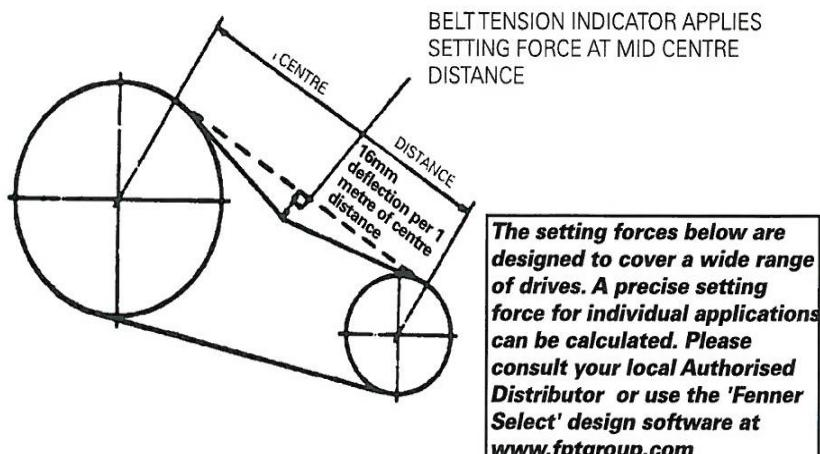
Also the tensioning of the belts is a major factor in the lifetime of the pulleys and belts. Incorrect tensioning can easily cause the belts to slip which then makes them brittle due to heat, which then wears out the pulleys.
