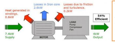
This is based on a 20kw motor running at 20% load.
