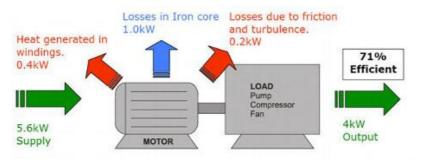
20kw motor running at 20% load with a FE Optimising soft start.
